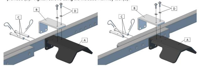
3. Secure Height Assist in place using the Pins <u>UNDERNEATH</u> the side extrusions. Secure pins using clips provided.
