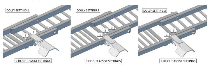
2. Depending on the location chosen, the Height Assist should be assembled to fit on top of either (1) side extrusion or (2) side extrusions. Attach Main Bracket (A) to Bracket 2 (B) using the button head screws and lock washers provided (D). Tighten screws using the included Hex Key tool (E).
